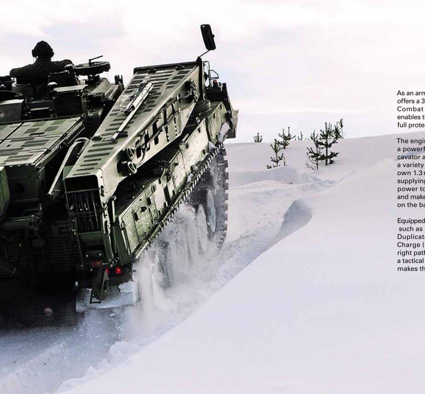
As an armoured recovery tank, the WiSENT 2 offers a 32-ton crane arm and a sophisticated Combat Recovery System (CRS), which enables the recovery of other vehicles under full protection.
