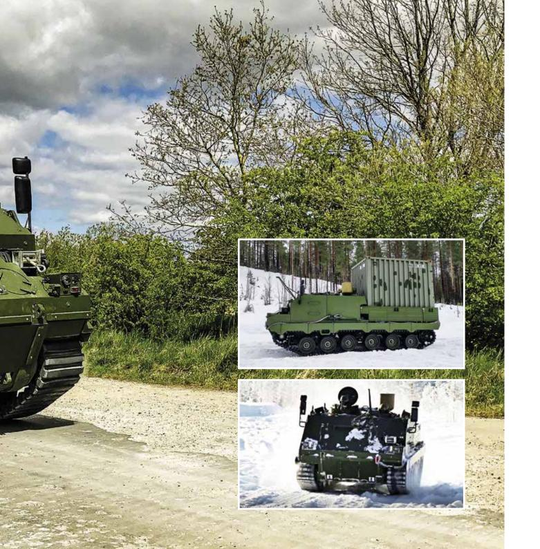
The ACSV G5 runs on a composite rubber track system which drastically reduces vibrations and noise, both inside and outside the vehicle. As a result, the rubber track reduces the strain on the equipment as well as on the soldiers inside the vehicle. The track contact length and the width of the track ensure very low ground pressure and guarantee excellent mobility on all surfaces, especially on snow, soft sand or boggy ground.
