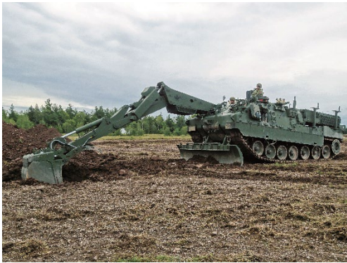
Fig. 3: The WiSENT 2 can be configured either as a recovery, engineer or mine-clearing vehicle or as a protected bridge-laying vehicle and is ideally suited for Leopard 2 user nations.
